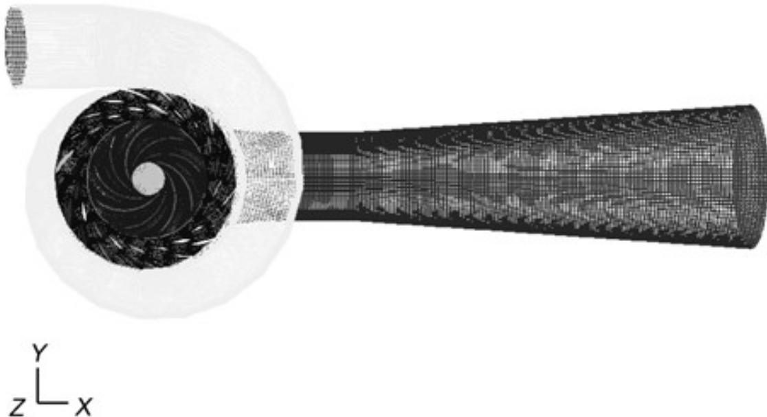
Figure 5. Mesh generation with different parts identified by different colours [6].
