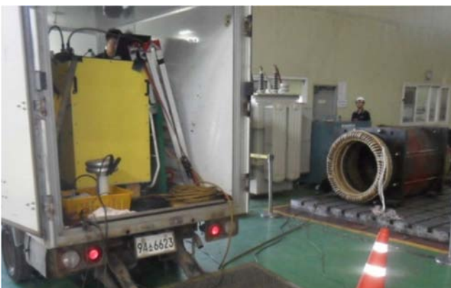
Figure 2. Insulation diagnosis test.
